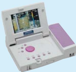
2D THERMO HITESTER 3460 performs 2-dimensional temperature measurement with a newly developed thermopile array sensor (8 $\times$ 8 elements), dividing the measured part of the visual image area into 64 boxes and displaying the temperature with a high-speed response of approximately 0.5 seconds.
