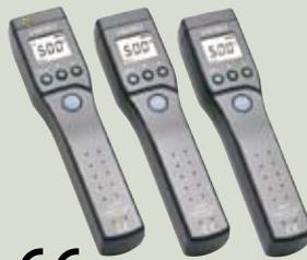
Long-range, narrow field (Ø72mm at 1m) model 3415-01 (with 2-beam laser marker) and model 3418 (without marker). Short-range spot measurement (Ø2.5 mm at 3 cm) model 3416-01. All are easy to operate and provide temperature readings at the touch of a button. Measurement range is -50 to +500°C, with a resolution of 1°C, and measurement time is 1.5 seconds.
