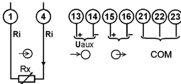
Picture 8c: Connection diagram 2-wire
