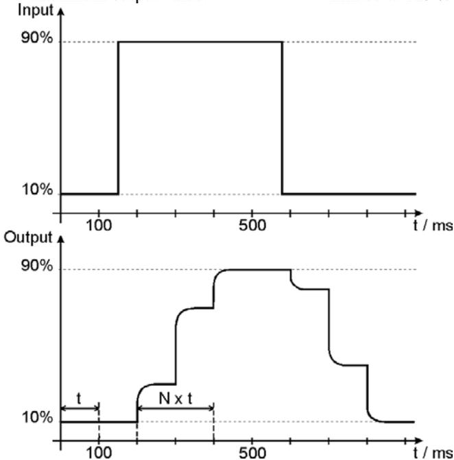
Picture 3: Output transfer characteristic
