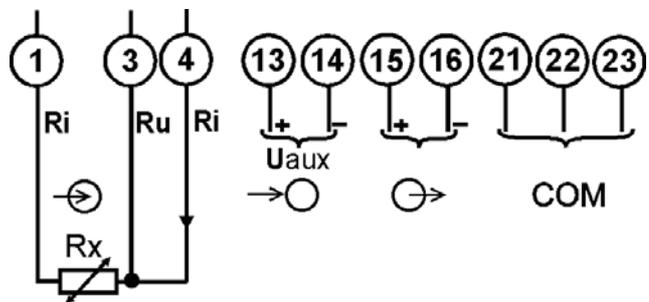
Picture 8b: Connection diagram 3-wire
