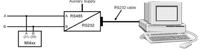
Picture 6: Connection of MI452 on RS485 communication line
