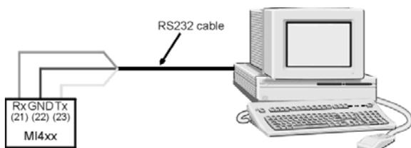
Picture 5: Connection of MI452 on PC via RS232 communication
