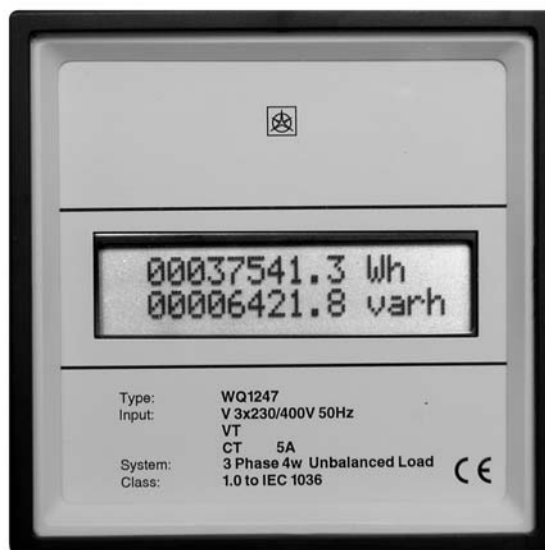
Picture 1: Energy Meter WQ1247
