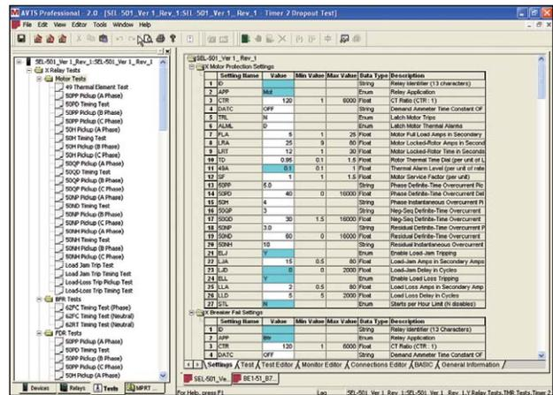
This example shows the organization tree descending by region, then substation, line, panel and finally the actual relay in the panel. The relays installed are then listed under that location. The heirarchical structure of AVTS includes up to 5 levels of organization.
