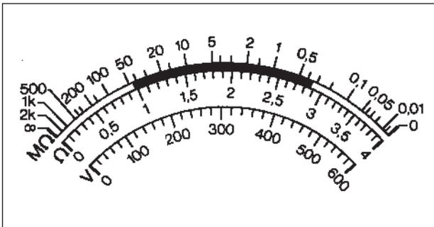
MJ10 scale is shown. BM12 scale is the same but has a battery condition indication mark added.
