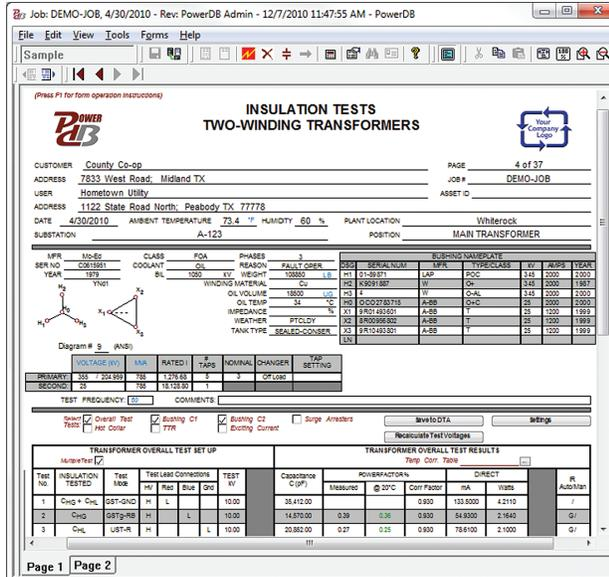
Figure 1: Data Entry & Automated Control of Megger DELTA Test Sets
