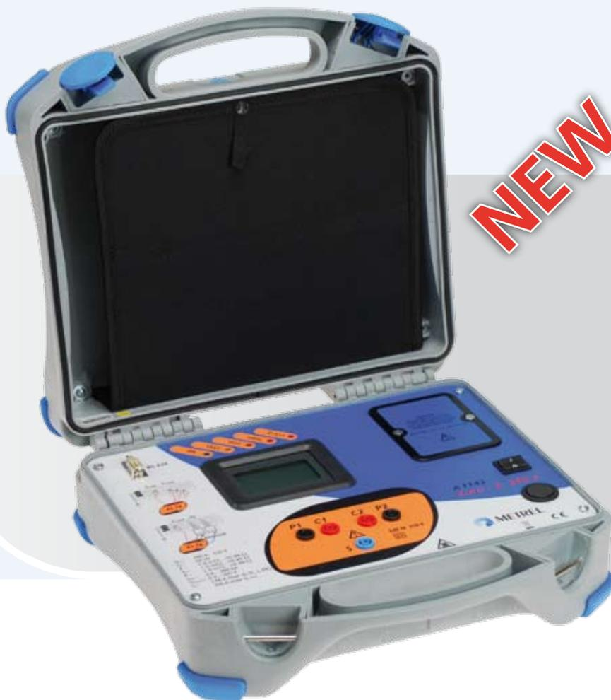
The **Euro - Z 290 A** is a professional portable test instrument intended for **low impedance measurements** in environments up to **CAT IV /310 V**. It can operate alone or in combination with the METREL instruments. **High precision line impedance** and **high precision fault loop impedance** measurements in range from 1 mΩ up to 19.99 Ω are its excellence.
