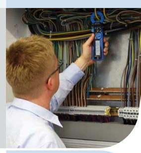
MD 9270 is a unique earth leakage clamp meter. It not just has the ability to accurately read the TRMS AC leakage current of a system, it can also detect losses in the system and suggest possible reasons for the loss. The voltage, power, harmonic, power factor (PF), total harmonic distortion (THD) and crest factor measurements make this instrument suitable for any electrician and engineer.
