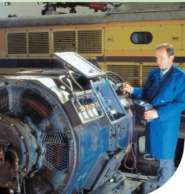
Advanced, field proven instrument. Technical demands require high performance measuring instruments capable of measuring polarization index (PI), dielectric absorption ratio (DAR), dielectric discharge (DD), insulation system capacitance. Easiness of use, high EM immunity and automatic discharge of load after completed measurement are just some of many outstanding features that distinguish Metrel HV testers from other similar products on the market.
