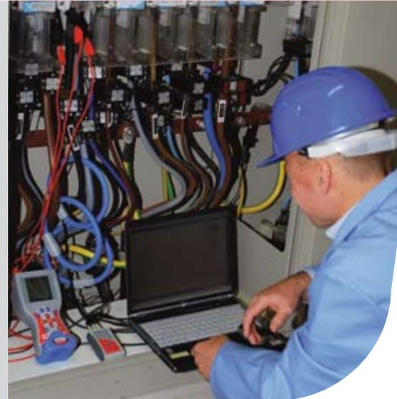
**PowerQ <sup>Plus</sup>** is a genuine, portable 3-phase power quality analyser which favorably competes with higher priced instruments and can be easily implemented in a variety of different situations.
