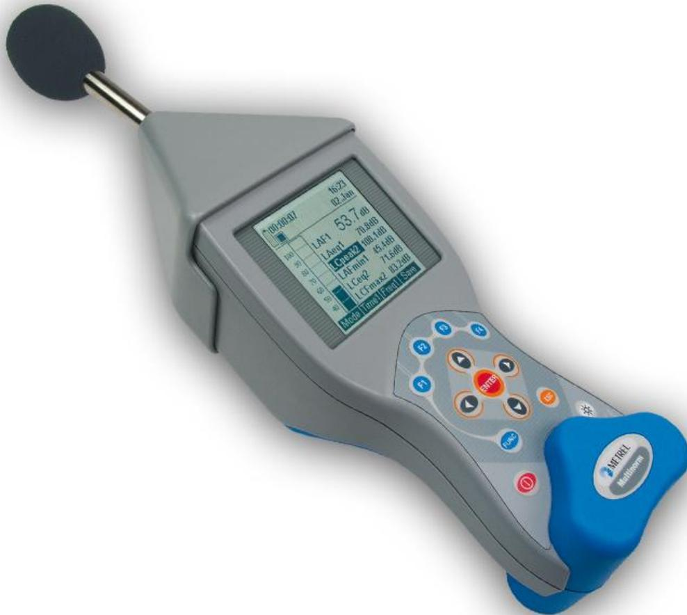
Universal all-in-one instrument for measurement of air temperature, air velocity, relative humidity, illuminance, luminance and the Class 1 (Pro Set) or Class 2 (Euro Set and Standard Set) sound analyses.
