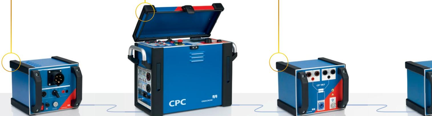
CPC 100 + CP RC1: testing GIS up to 123 kV rated
