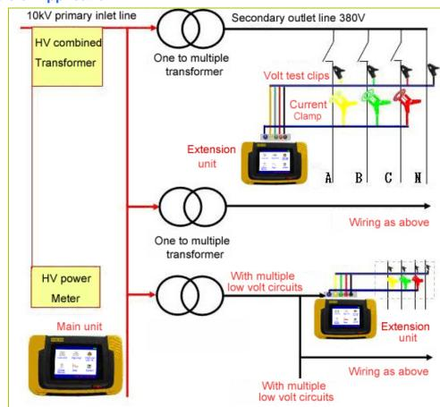
This is application in high-volt metering unit with multiple units working simultaneously. It is also applicable in other metering units and power meters.
