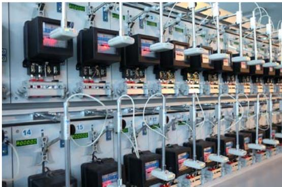
PITE 9153 series are meter test equipments that can measure all types of single phase mechanical meters, electric mechanical meters and electronic meters of class 0.5 or lower. It adopts operation ways of automatic semi-automatic, or manual measurement. With different options for standard referenced meter and power amplifier, PITE offers different models of different accuracy to meet various customers' need for power meter calibration.
