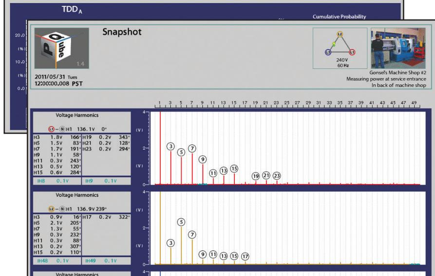
**A "harmonic profile" snapshot.** Identify exactly which harmonic is causing problems. Harmonic snapshots can be generated from the PQube on demand, or every 10 or 15 minutes (user-selected).
