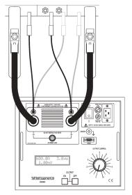
the current to the desired level, and switch the output off. The readings will be held on the display.
