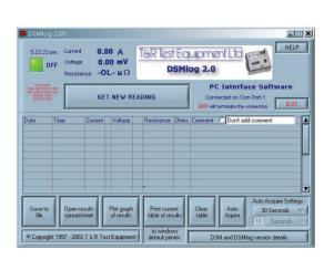
The DSM600 is simple to operate, only requiring the user to switch the output on and set the test current. Selection of all ranges is fully automatic, and current, voltage and resistance are displayed simultaneously at all times. The resistance is calculated from the test current and sense voltage, and there is no need to set an exact test current to guarantee an accurate test result. To assist the user, all readings are held on the display when the output is switched off.
