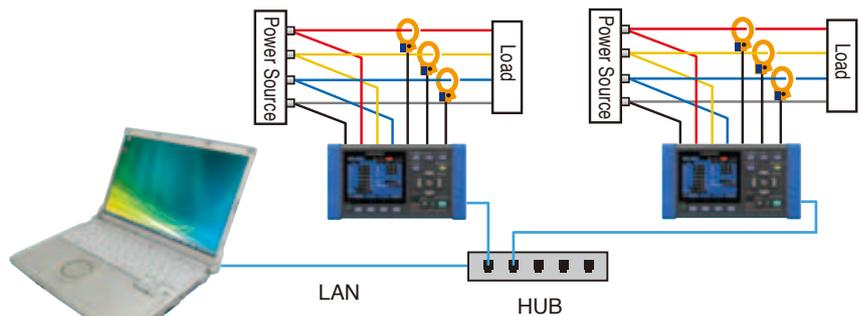
Files recorded in the Clamp On Power Logger's internal memory or SD card are accessible via a LAN or USB connection, and are downloadable using the free **PW3360 Setup and Download Software**.
