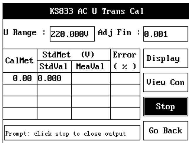
Figure 75 AC Voltage Transducer Inspection interface
