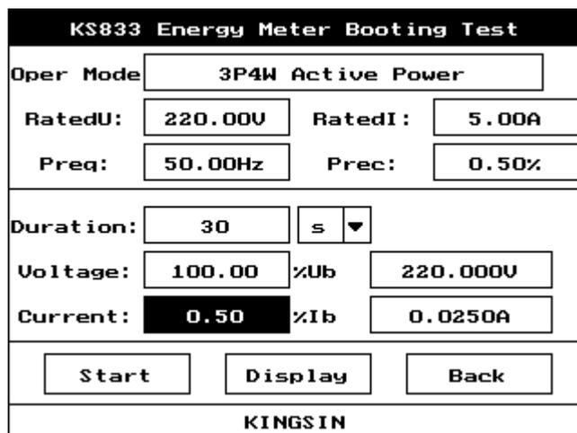
Figure 58 Booting tests of electrical energy meters
