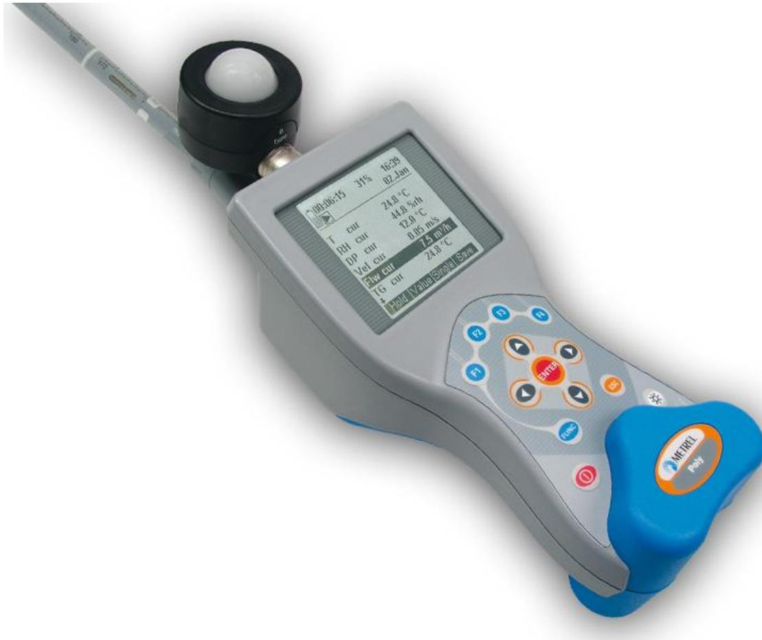
Measurement functions for air temperature, air velocity, relative humidity, illuminance and luminance are all found within one device.
