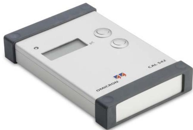
Calibrating the test circuit is mandatory prior to measurements when they are carried out in accordance with IEC 60270. To do this, a defined charge is injected into the test set-up using the CAL 542 and the MPD system is calibrated to this value.
