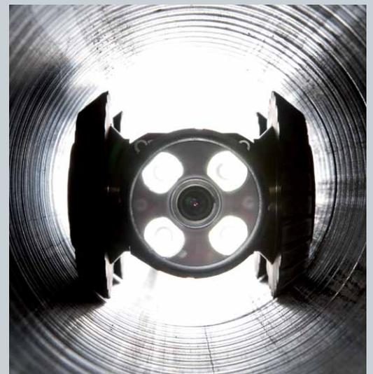
operate fully submersed and are water resistant to depths of up to 100m (330'). They are constructed from brass and stainless steel and are built with a single or twin 50W motor configuration, powerful enough to move through almost any pipeline system. The integrated sensitive inclinometer and the multi-frequency sonde allow you to map pipeline topography easily and efficiently.
